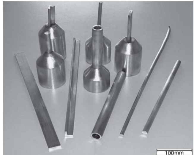
Fig. 10 Received extruded profiles and reminders worked at low temperature. The surface of the material is affected neither by hot nor cold cracks. This is also valid for other profile dimensions, which were not the subject of this article.
